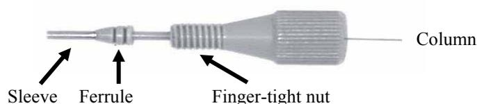
Fig. 3: Fitting connection
