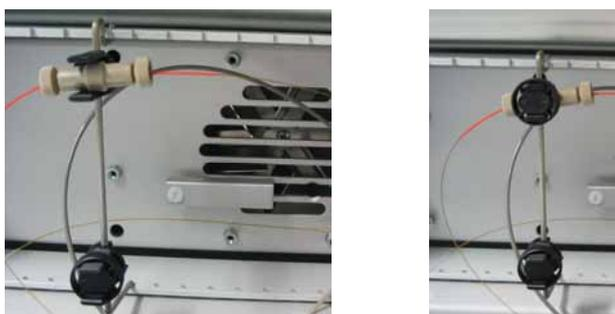
Fig. 18: Column installed in the clip
